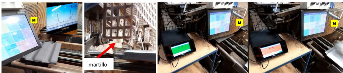
Fig. 8: Industrial line test with the hammer, FFT spectrum or QC software screening (Green/Red)
