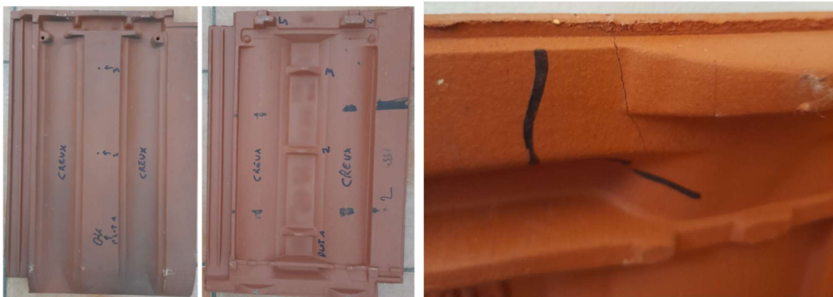
Fig. 3: Front and back of the studied model (note valleys, lugs, grooves). "Crack" defect
