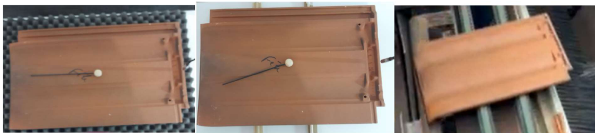
Fig. 5: Tile learning protocol: (A) "free", (B) "captive on bars", (C) on the industrial line
