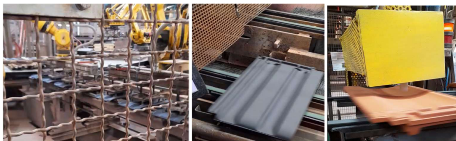
Fig. 11: (a) Line configuration with unloading robot and (b) bars 14 cm apart; (c) configuration with bars 25 cm apart
