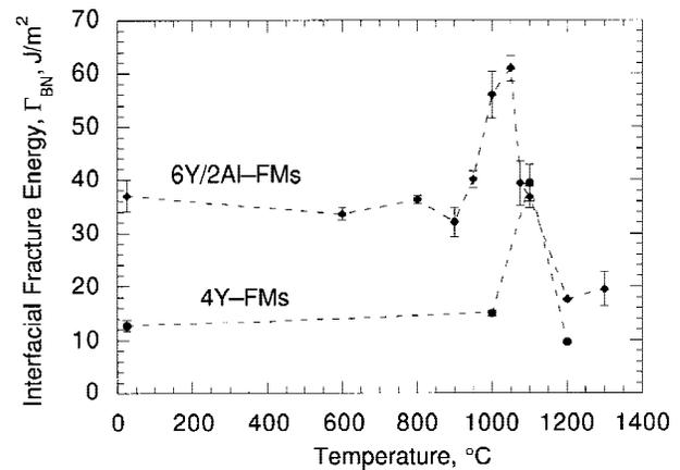
**Fig. 7.** Plot of  $\Gamma_{BN}$  for both compositions of fibrous monoliths studied. 6Y/2Al-FMs exhibited a sharp increase in  $\Gamma_{BN}$  between 1000° and 1050°C. The interfacial fracture energy peak in 4Y-FMs was shifted to 1100°C.
