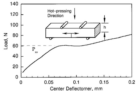
**Fig. 1.** Typical results from a Charalambides interfacial fracture energy test. These data were taken from a specimen tested at 1200°C. The schematic shows the notched beam and the interfacial crack.
